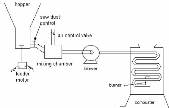
Figure 1: Schematic of the Sawdust Combustor with Accessories
