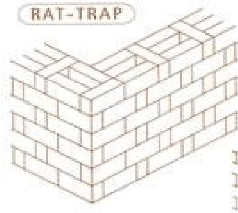
Figure 2a. Schematic of Rat Trap Bonding
